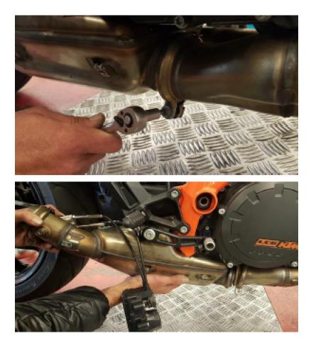
(d) Remove trains and the plate of the actuator. To do so please secure disk using a wrench or pliers in order to prevent the motor from being damaged.
