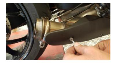
b) To remove the exhaust valve actuator, first release the brake fluid reservoir and secure it nearby so it will remain in the vertical position. Then pull out the connector plug on the motor and remove the motor (a screw on the front and three screws on the back.
