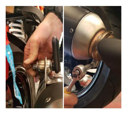
Carefully remove the gasket from the original front silencer. This must be used
